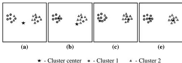
Notes: (a) Represents the original image with the different patterns and the centroid of the image data; (b) illustrates the cluster membership after the first iteration; (c) shows the cluster membership after the second iteration; (d) represents the final clustered image
