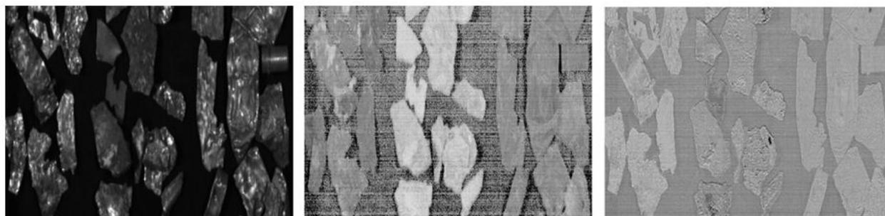
**Figure 9** Results achieved after the application of intensity correction. (a) Raw hyper-spectral data. (b) Stockman and Gevers [33] intensity correction. (c) Montoliu et al [34] intensity correction.
