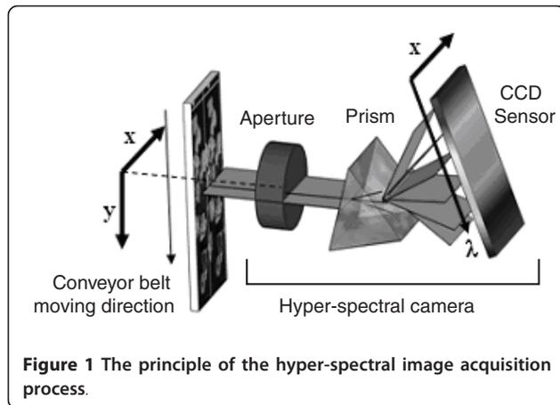
**Figure 1** The principle of the hyper-spectral image acquisition process.
