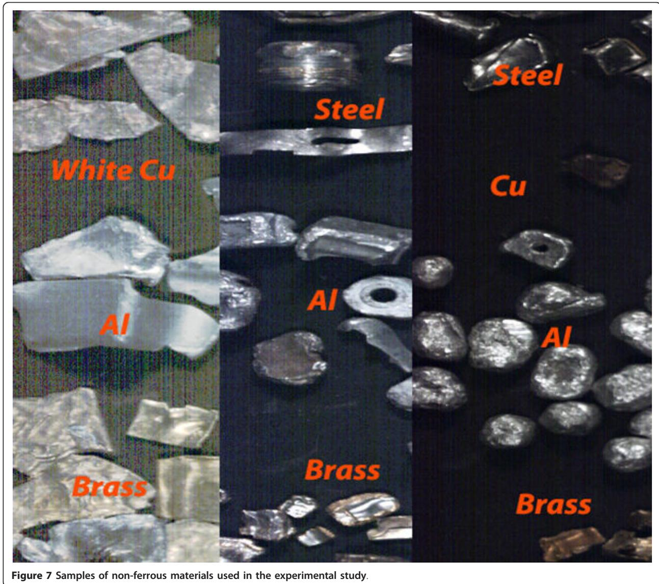
**Figure 7** Samples of non-ferrous materials used in the experimental study.
