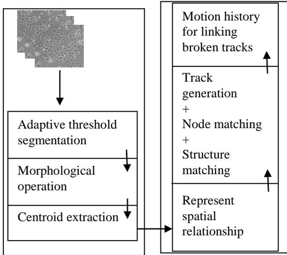
Figure 2. Flow diagram of the proposed tracking framework. Left – Centroid extraction module. Right – Tracking module
