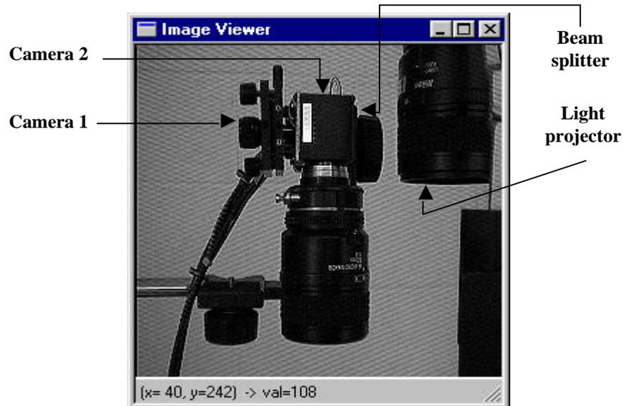
Figure 4: The 3-D sensor and its principal components.
