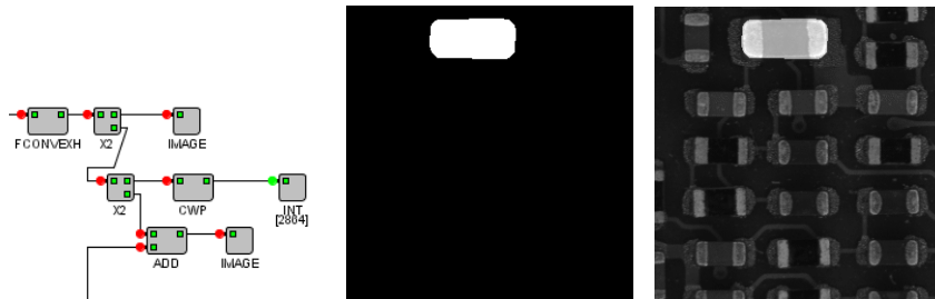
Figure 14: Identifying calculating the area of the largest component. Overlay on original image to highlight its location.
