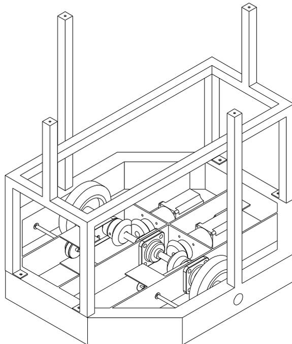
Fig. 3. Model of assembled drive and chassis components.
