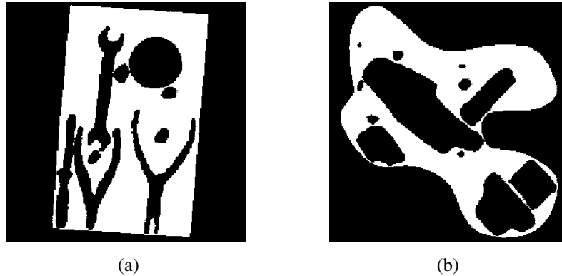
Figure Z.7. Packing items into defective regions. (a) Packing tools into a defective tray. (b) Cutting jacket template pieces from a fabric segment, which contains defective regions
