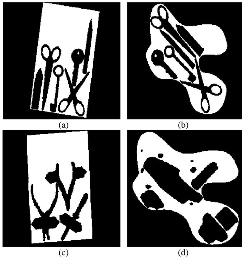
Fig. 2. Automated packing of irregular shapes. (a) A rectangular tray. (b) An irregular scene. (c) Allowing for robot gripper considerations. (d) Cutting jacket template pieces from an irregular fabric segment which contains defective regions.
