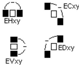
Figure 2: The four local discontinuity detectors of the Adaptive filter
