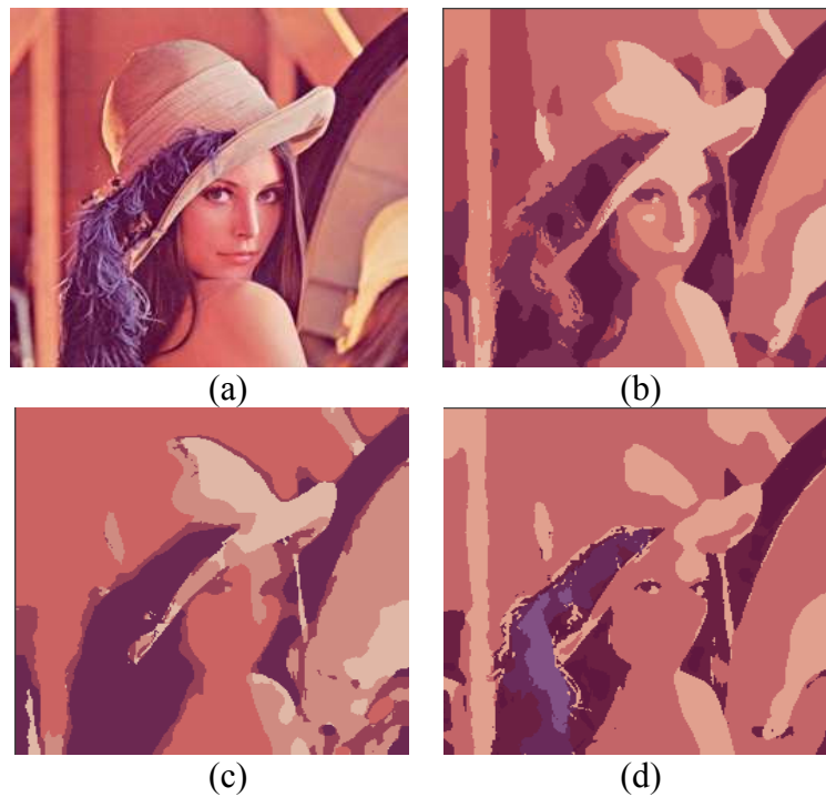
Figure 5. Segmentation results. (a) Test image. (b) Segmented result – RGB color space. (c) Segmented result – YIQ color space. (d) Segmented result – HSI color space.
