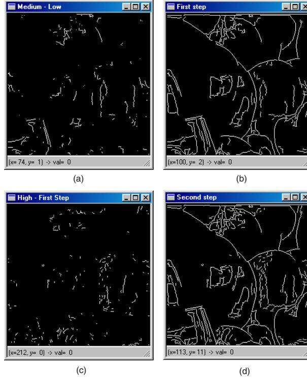
Figure 3. The edge reconstruction process for images illustrated in Figure 2. (a) The subtraction of the low edge density image from the medium edge density image. (b) The resulting image after first iteration. (c) The subtraction of the resulting image from the high edge density image. (d) The output image.
