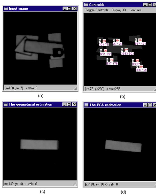
Figure 12: Recognition results when the system is applied to a scene containing clutter and occlusion. (a) The input image. (b) The resulting image data. (c) The topmost recognized region. (d) The pose estimation for the topmost object.
