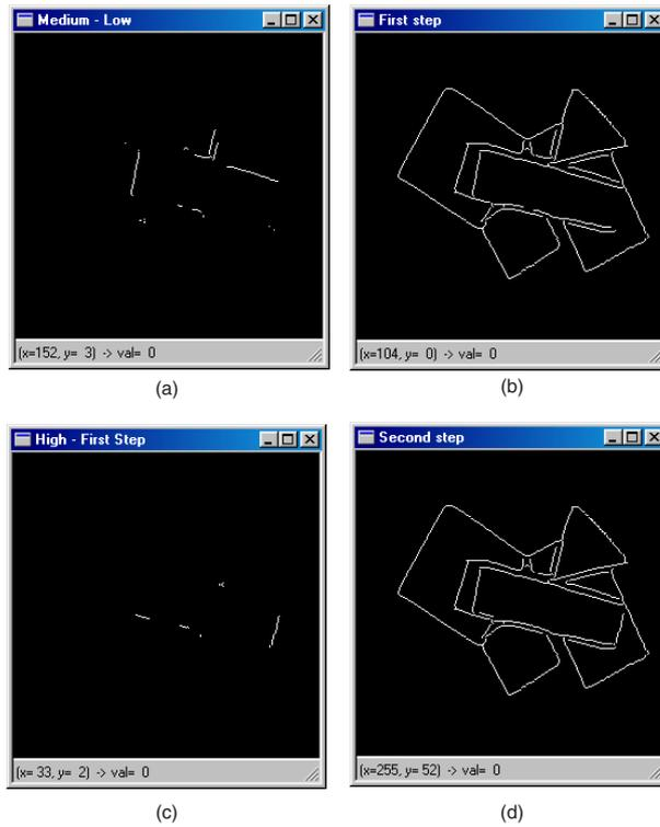
Figure 6: The edge reconstruction process for images illustrated in Fig. 5. (a) Difference between the medium and lowest resolution images. (b) The resulting image after first iteration. (c) Difference between (b) and the highest resolution image. (d) The output image.
