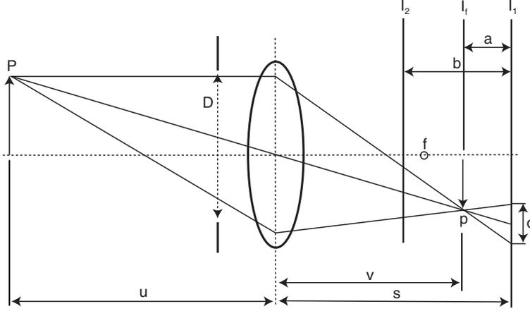
Figure 2: The image formation process. Depth is determined by measuring the relative level of blurring.
