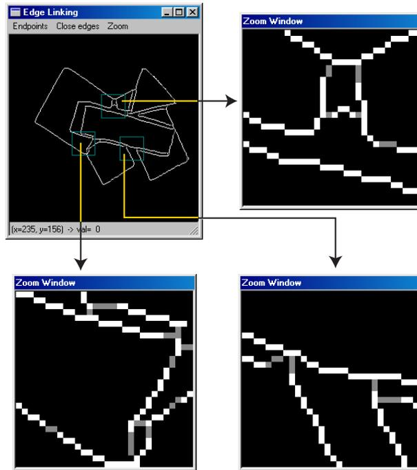
Figure 7: The edge linking results when the algorithm is applied to the image illustrated in Fig. 6(d) (linking pixels are shaded).
