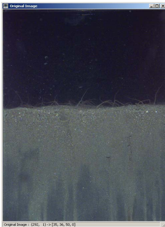
Figure 5. Detection of the oxidised layer. (a) Original image (sample Marg1). (b) Oxidised layer.
