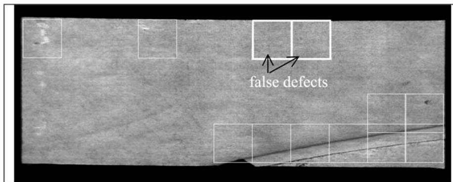
**Note:** The white box is drawn around  $128 \times 128$  pixel image sub-sections considered to be defective. True positive defects are correctly detected as indicated by the faint boxes
