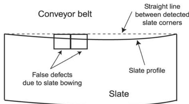
**Figure 7** False defect generation due to depth profile variation
