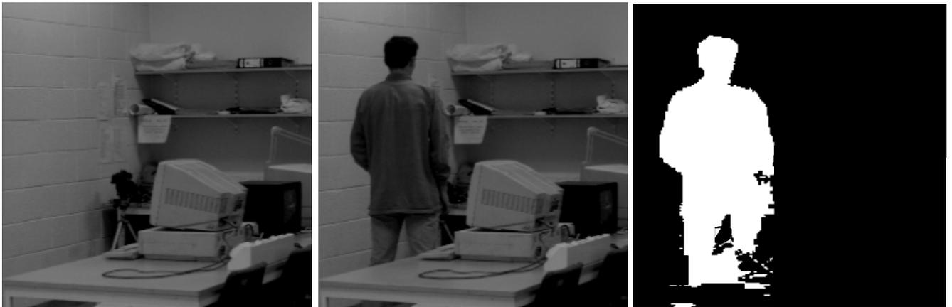
Figure 5. Showing the reference image, the image with the object and the extracted results.
